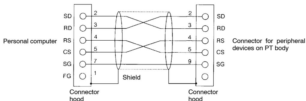
**Note** Connect the shield wire to the connector hood at both the personal computer and at the PT.
