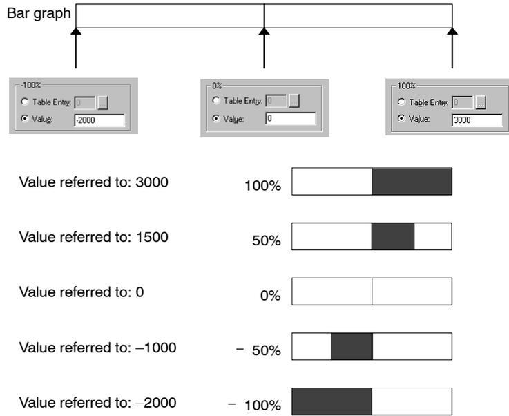
If the 100% value, 0% value, and -100% value are set using numeral memory table entries as indicated below, the percentage value of the reference value is calculated according to the value stored at the specified address.
