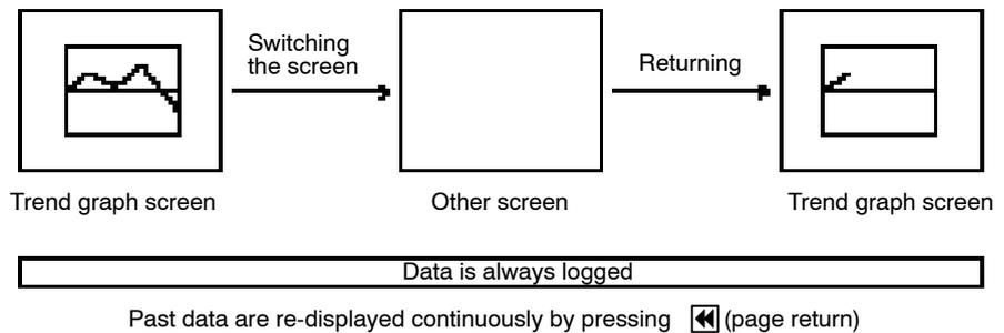
Although the trend graph starts displaying new data when the screen is switched back to the trend graph display screen, it is possible to display the data of the period during which the trend graph was not displayed by pressing a touch switch that has the function to display the past data.
