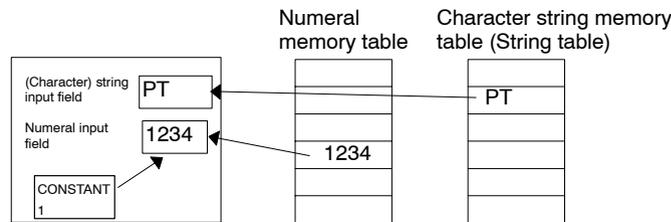
By setting the setting data to a memory table entry or a touch switch beforehand, the data is copied to the input field at the cursor location as desired.
