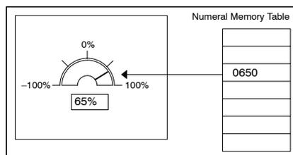
A value in a numeral memory table entry is converted into a percentage value, in the range from 0 to 100% or from -100% to 100%, and displayed in the form of quarter, semicircle, circle graph. Also, scale display is available.
