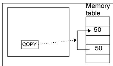
(1) When a touch switch is pressed, the data in the memory table entry or a constant is copied to another memory table entry or input field.
