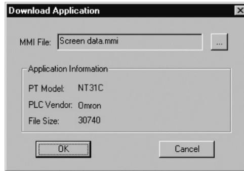
If the PT is not in the Transmit mode, a timeout error occurs in about 10 seconds at the NT Transfer Utility. In this case, set the PT in the Transmit mode and click on  in the error message dialog box.
