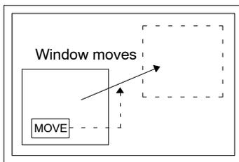
(1) When a touch switch (window move touch switch) is pressed, the window can be moved by touch panel operation at PT. When you press the destination (center of the window will come here), window will be moved to that position.
