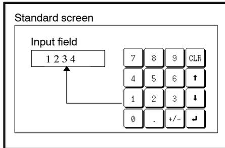
(1) When a touch switch is pressed, the input processing of the control code is executed as shown below.
