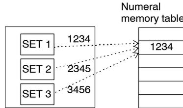
By setting a constant in the data setting field of a copy function touch switch beforehand, the necessary data can be copied to a numeral memory table entry as desired.
