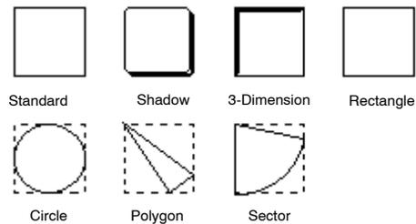
Although [Standard] and [Rectangle] have the same shape, how the touch switch frame is defined differs between them. With [Standard], the touch switch frame itself provides the display graphic. With [Rectangle], however, a rectangle shape can be specified independently of the touch switch frame and the touch switch frame can be separated from the rectangle shape.
