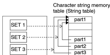
By setting the data in several memory table entries beforehand, the necessary data can be copied to the work area as needed.
