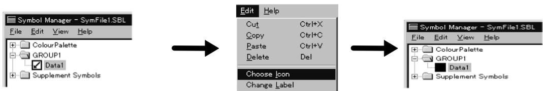
**Reference:** For an icon, 16×16-dot, 8-color bit map data can be used. Although bit map data larger than 16×16 dots can be used, only the 16×16 dots at the upper left area of such data is used.
