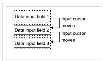
(1) When a touch switch (cursor moving touch switch) in an input field is pressed, the cursor moves to that input field.
