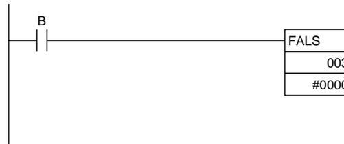
When input condition B goes ON, an error with FALS number 3 is generated and A401.06 (FALS Error Flag) is turned ON. Program execution is stopped.
