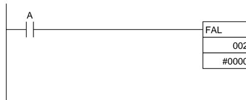
When input condition A goes ON, an error with FAL number 2 is generated and A402.15 (FAL Error Flag) is turned ON. Program execution continues.
