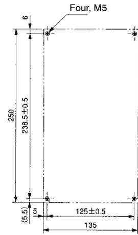
● Front Panel Mounting (Using Mounting Brackets)
